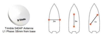
The Primary Antenna (Antenna 1) should be nearest to the sonar so that offset measurement errors are minimized. The Secondary Antenna (Antenna 2) should be a fixed distance from Antenna 1. It is recommended that the antennas be at least 2m apart. The antennas should be positioned parallel to the water surface to within 2-3cm.
